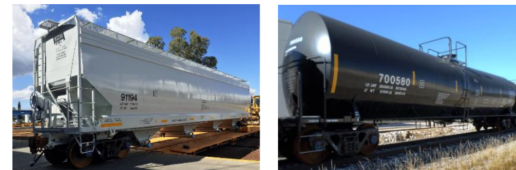
▲ Railcars (left: covered hopper, right: tank car)
