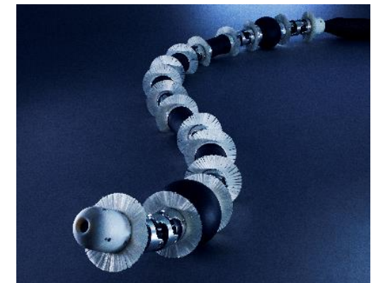
4 Sooha, an in-pipe crawling robot that mimics the movement of an earthworm, provided by SoLARIS.
