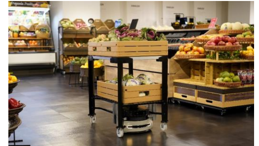
📷 2 A sample image of a conveyance unit installed on Armo, a robot under development
