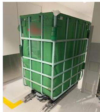
An indoor transport robot for hotels, etc.
