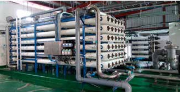
Seawater desalination RO system of the same size as that to be delivered
